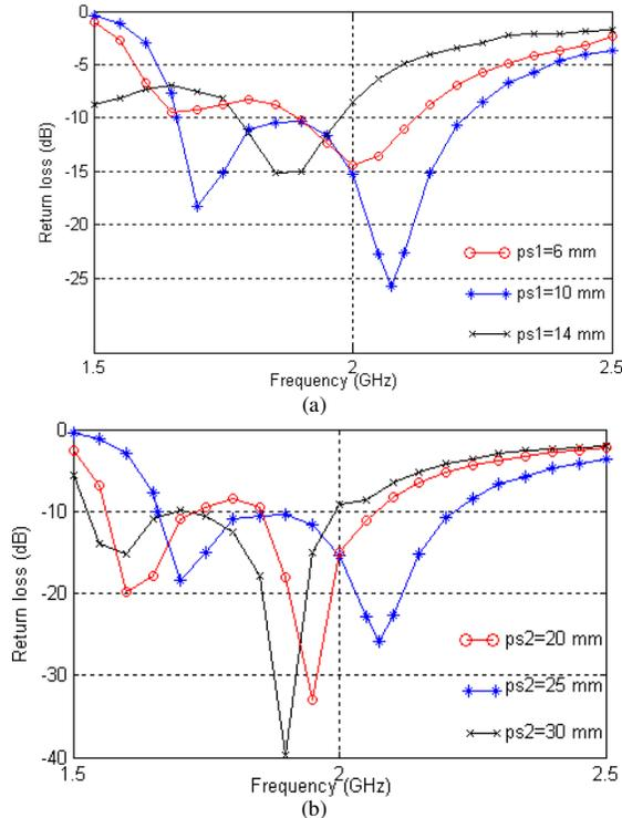
Figure 4. Calculated  $S_{11}$  of Comb-shaped antenna with different slot positions. (a) Effect of inner slot position. (b) Effect of outer slot position.
