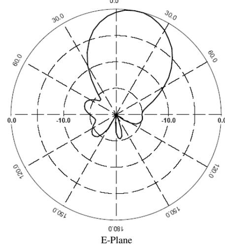
Figure 7. The E-plane and H-plane radiation patterns of proposed comb-shaped antenna.
