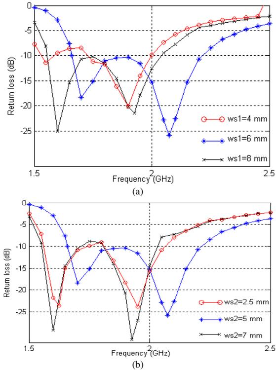
Figure 3. Calculated  $S_{11}$  of Comb-shaped antenna with different slot width. (a) Effect of inner slot width. (b) Effect of outer slot width.
