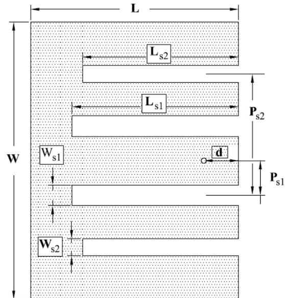
Figure 1. Geometrical configuration of the proposed comb-shaped antenna.
