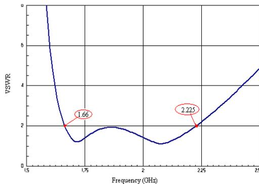
Figure 5. The curve of VSWR for proposed wide-band antenna with dimensions presented in TABLE I.
