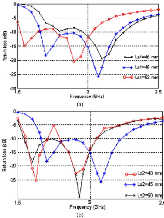
Figure 2. Calculated  $S_{11}$  of Comb-shaped antenna with different slot lengths. (a) Effect of inner slot lengths. (b) Effect of outer slot lengths.
