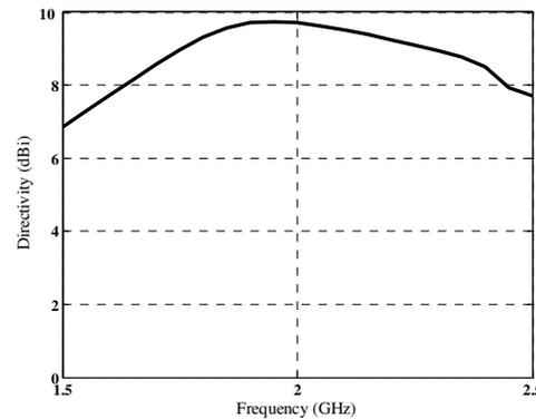
Figure 6. The calculated directivity of the proposed comb-shaped antenna.
